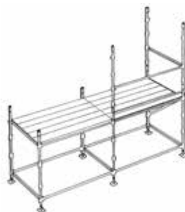
Prefabricated scaffold (modular type)
